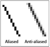
Figure 17-4: An aliased line and an anti-aliased line.
