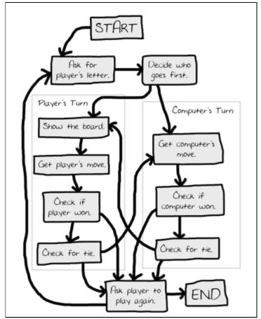
Figure 10-1: Flow chart for Tic Tac Toe
